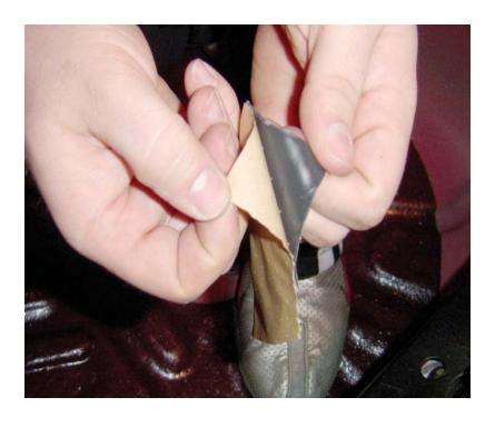
2. Remove the paper backing to expose the adhesive.
